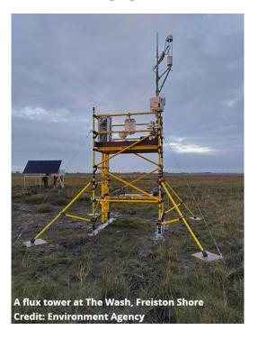
A flux tower system is being installed on site this week. Flux towers measure the exchanges of carbon dioxide, water vapor, and energy between plants and the atmosphere.
