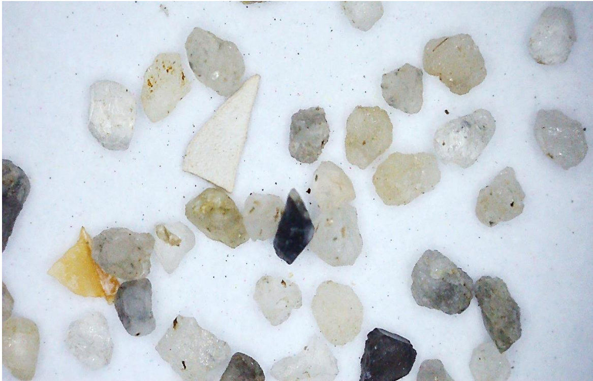
Figure 21. Close up of sediment grains retained on the 500µm sieve at site P5-MID.
