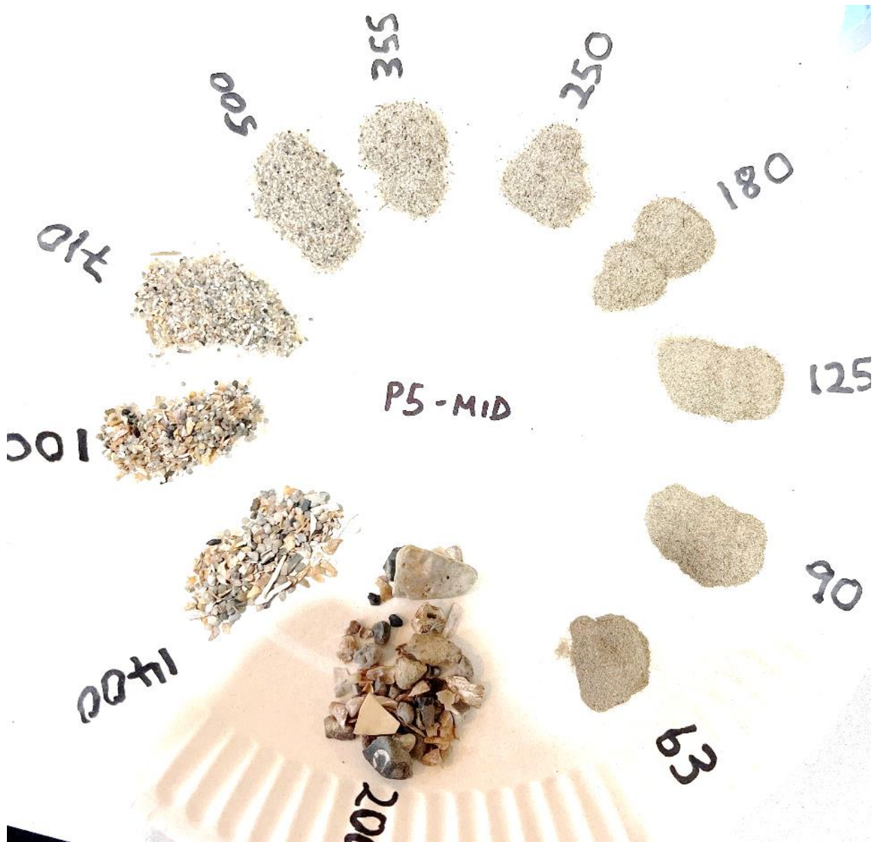
Figure 20. Grain size fractions >63\mu\text{m} for site P5-MID, on the shoal in the mid-channel central region.
