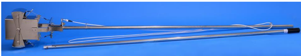
Figure 5. Pole mounted Ekman grab used during the survey (2m length, corer size 20 x 20 x 20cm).
